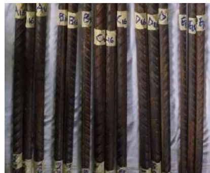
Figure 3.2: 16mm Rebar samples grouped based on the company
