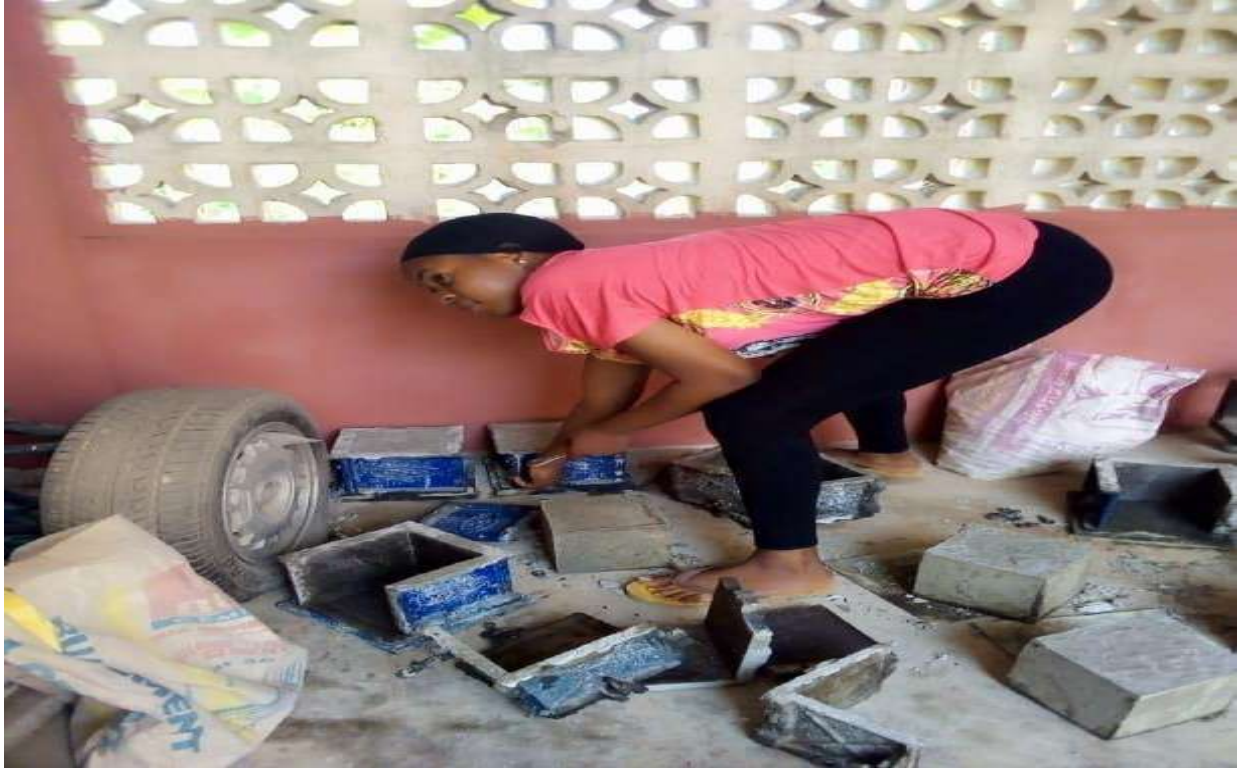
Plate 5: Getting Cubes Ready for Curing.
