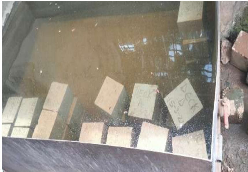
Plate 3.8: Curing of concrete cube specimens
