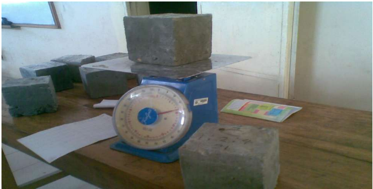
Plate 3.7 Weighing process to determine densities of concrete samples
