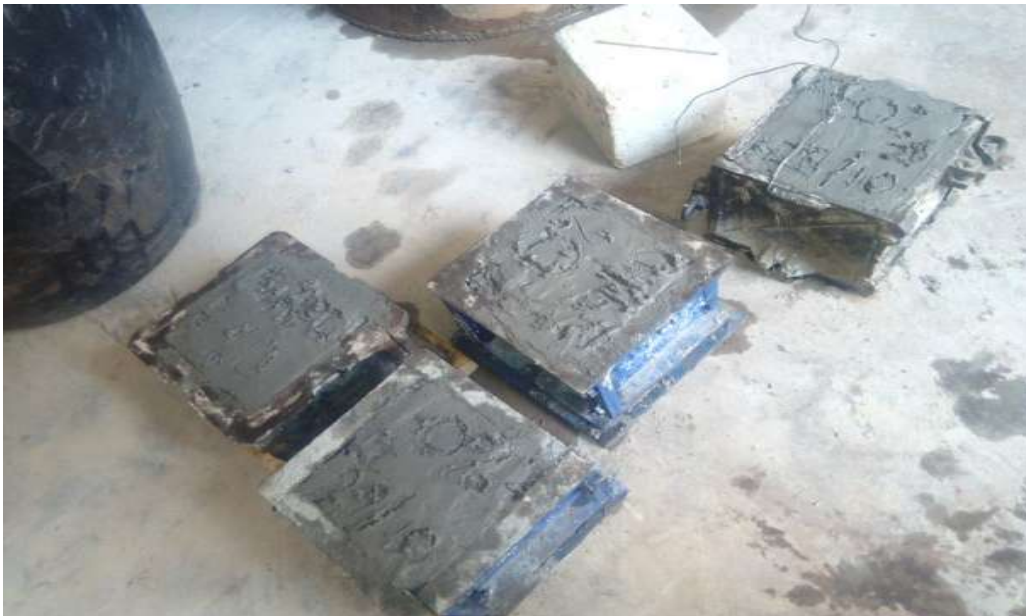
Figure 3.8: Concrete moulds filled with fresh concrete
