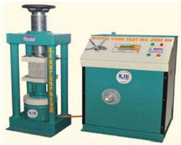
Fig 2.2a Compressive testing m/c cube.
