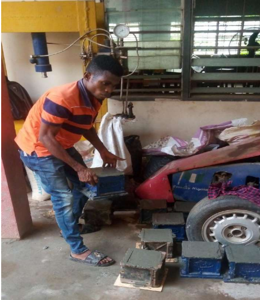
Plate 3.5 casting of concrete cubes
