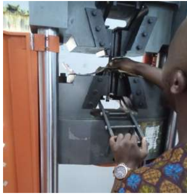
Figure 3.5: Placing and gripping the Sample on the machine
