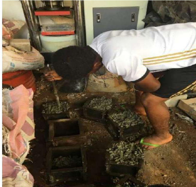
Plate 3.3: Tamping of concrete with a tamping rod.
