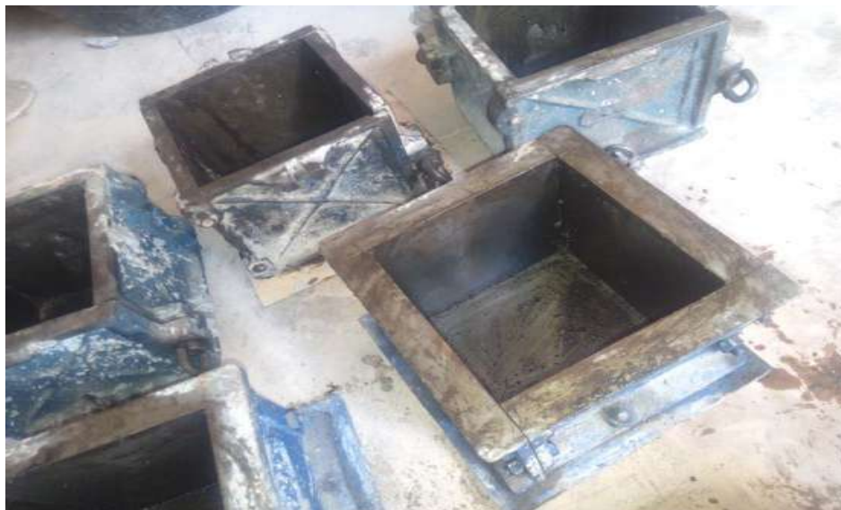
Figure 3.5: Metallic mould for concrete casting
