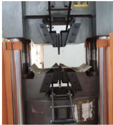
Figure 3.6: Fractured test sample in the UTM
