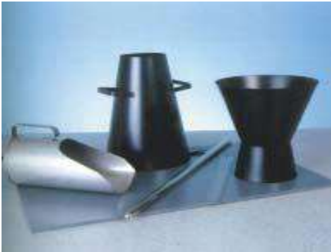
Plate 3.8 Apparatus used for Slump Test
