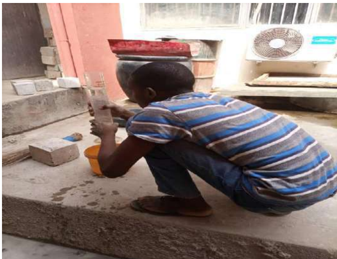
Plate 3.16: Measuring of water with the measuring cylinder
