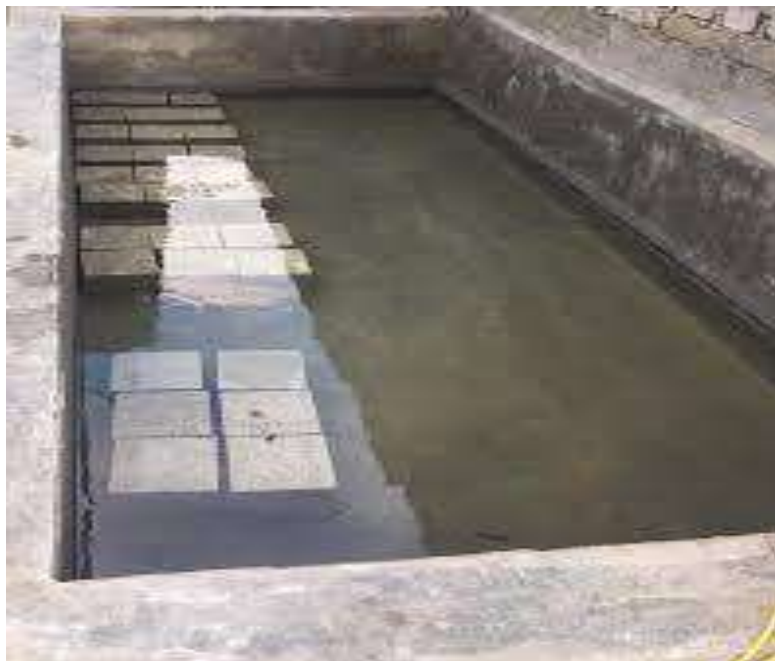
Plate 3.9 Picture of concrete cube curing tank.
