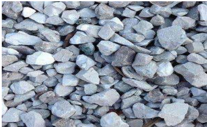
Plate 3.2: Coarse aggregate (crushed granite)
