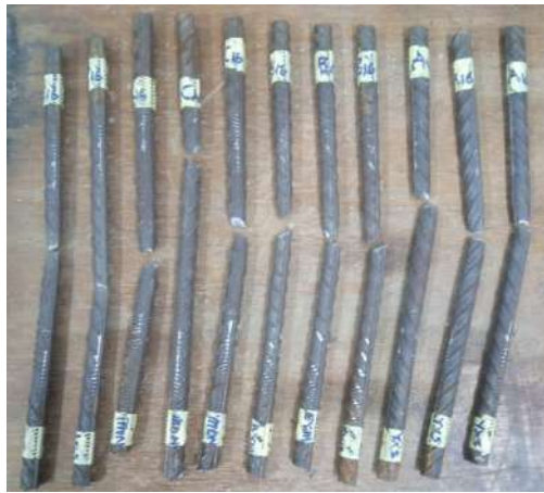
Figure 3.7: Fractured 16mm test samples
