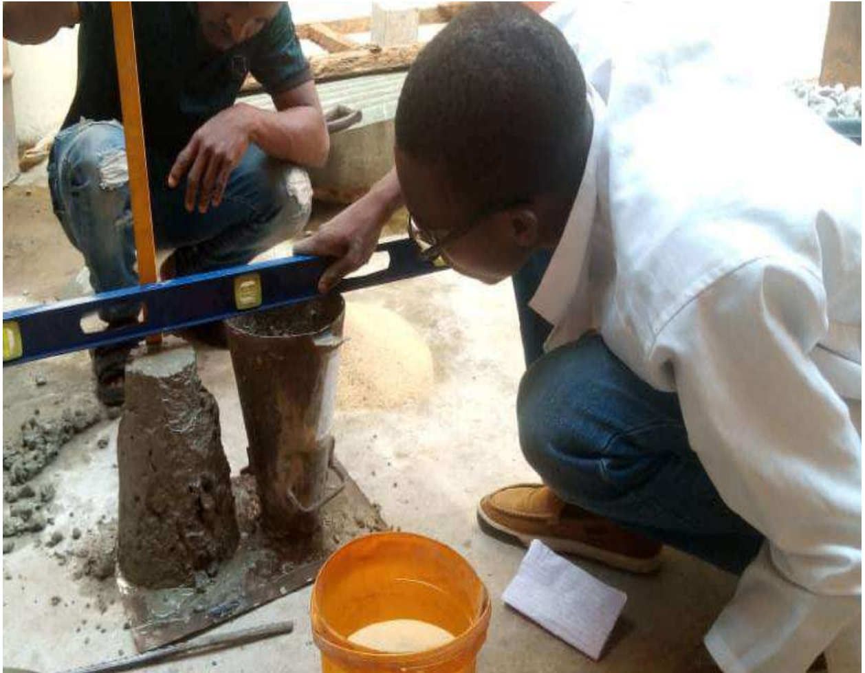
Plate 3.9: Slump Test on-going
