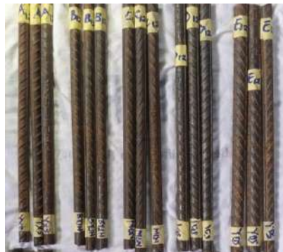
Figure 3.1: 12mm Rebar samples grouped based on the company
