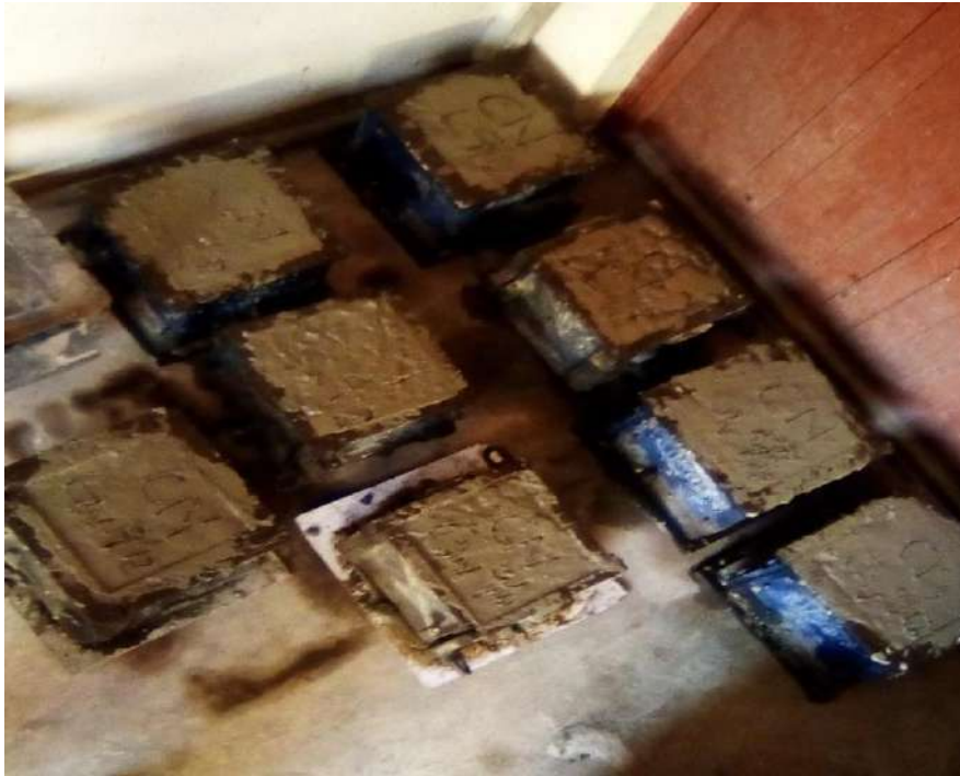
Plate 3.13: Concrete with mould
