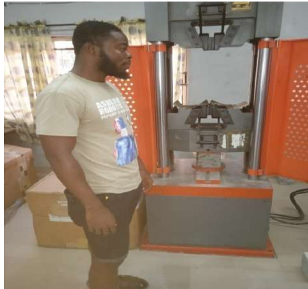
Plate 3.9: Crushing of concrete cubes with compressive test machine
