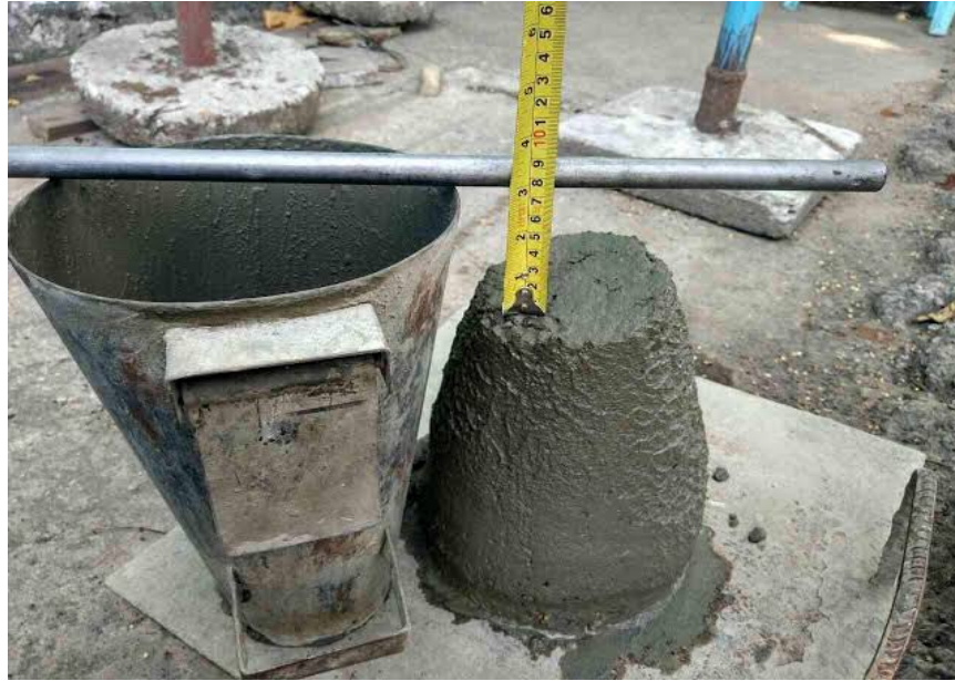
Plate 3.6: Measuring slump value
