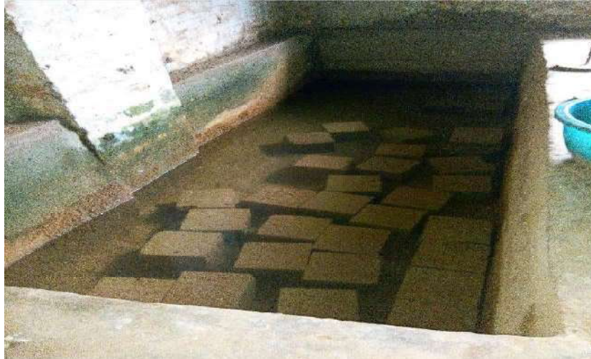
Plate 3.4: Curing of concrete cubes.
