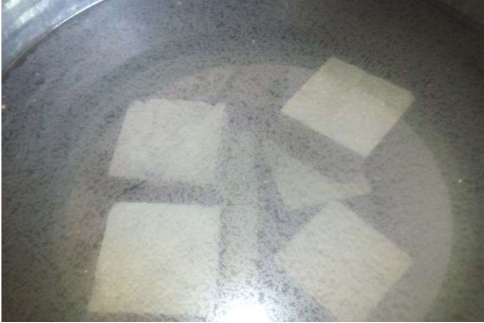
Figure 3.10: Concrete cubes in a concrete water tank
