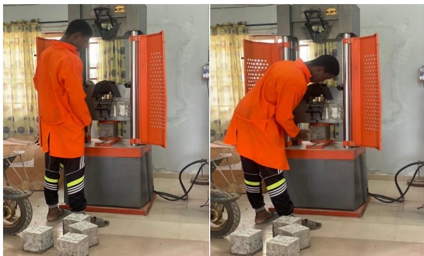
Figure 3.3. Crushing of Concrete Cubes
