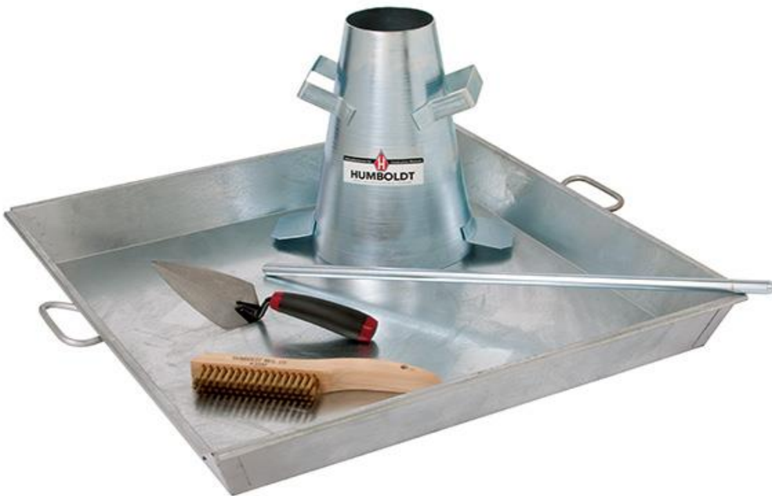
Plate 3.8 Apparatus used for Slump Test
