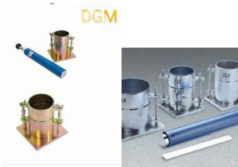
Plate 3.7 Apparatus employed for Compaction Test.
