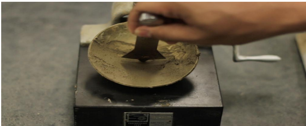
Plate 3.6: Cutting a groove at the middle of the soil paste with a standard grooving tool
