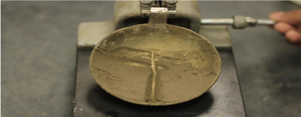
Plate 3.7: The groove at the middle of the soil sample before the application of the blows
