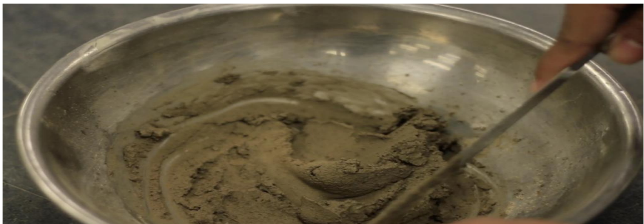
Plate 3.4: Preparation of soil slurry
