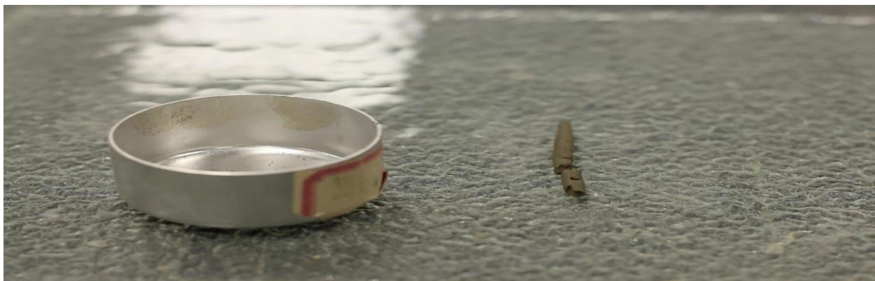
Plate 3.10: A sample thread of 3mm in diameter
