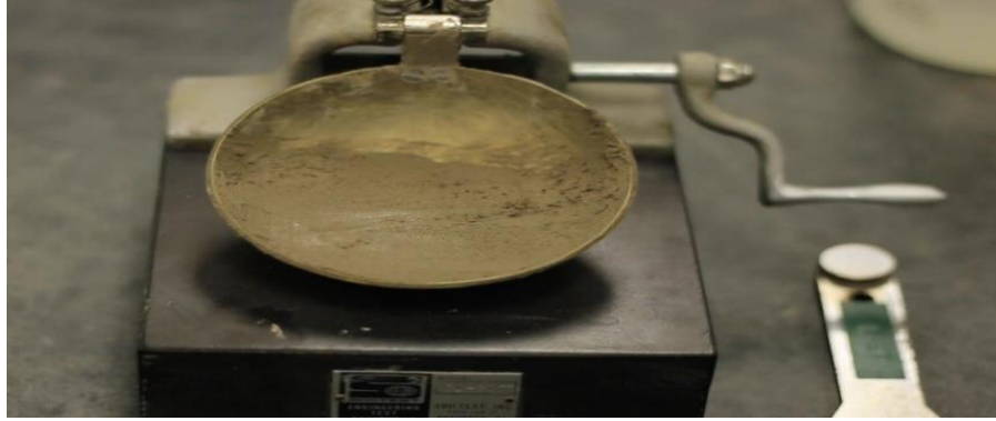
Plate 3.5: Placing the soil paste on the Casagrande apparatus
