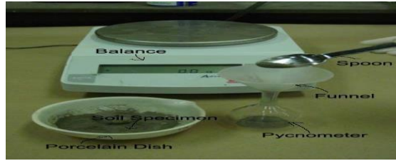
Plate 3.3: Apparatus used for Specific Gravity Test
