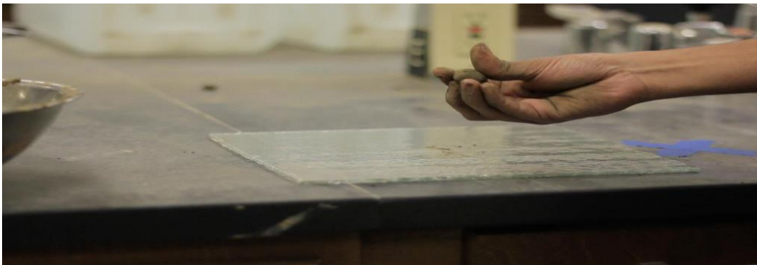
Plate 3.9: Sample preparation for the plastic limit test
