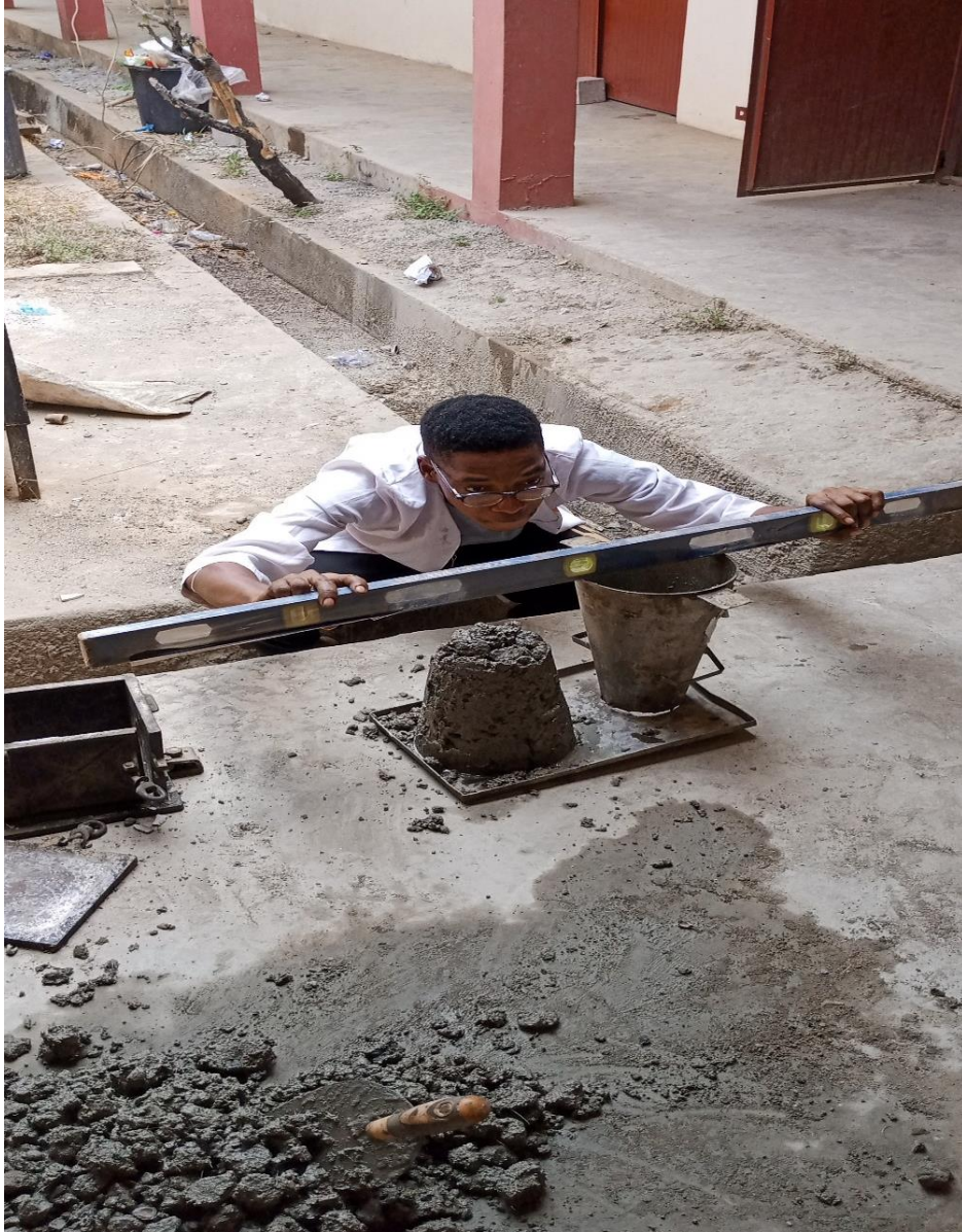
Figure 3. 7 Measurement of slump.
