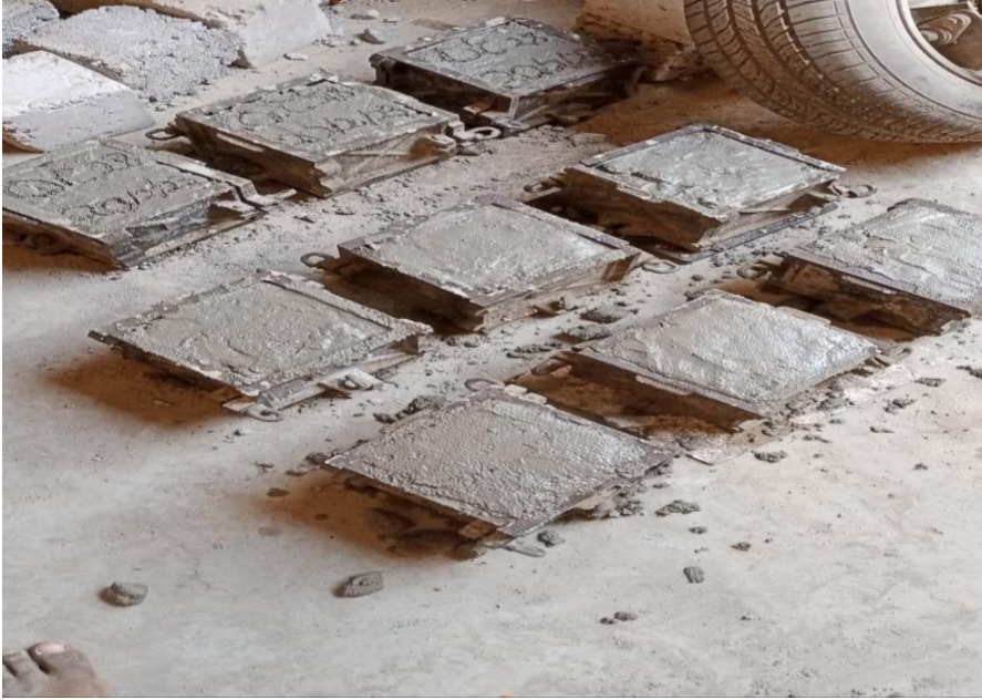
Figure 3. 3 Concrete cubes in mould
