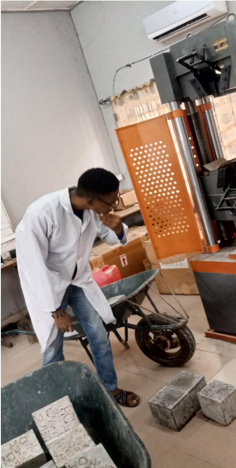
Figure 3. 4 Crushing of the concrete cubes
