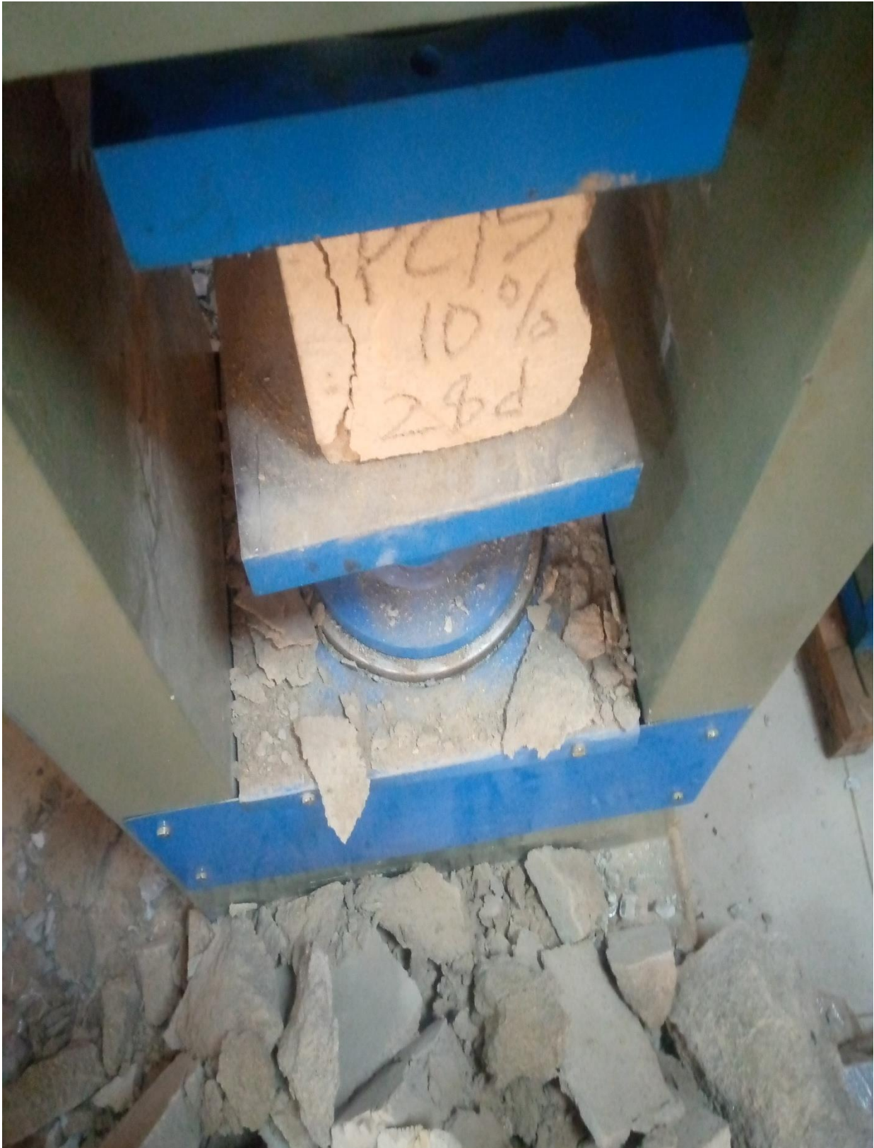
Fig 3.3: crushing of blocks using the compressive strength machine.
