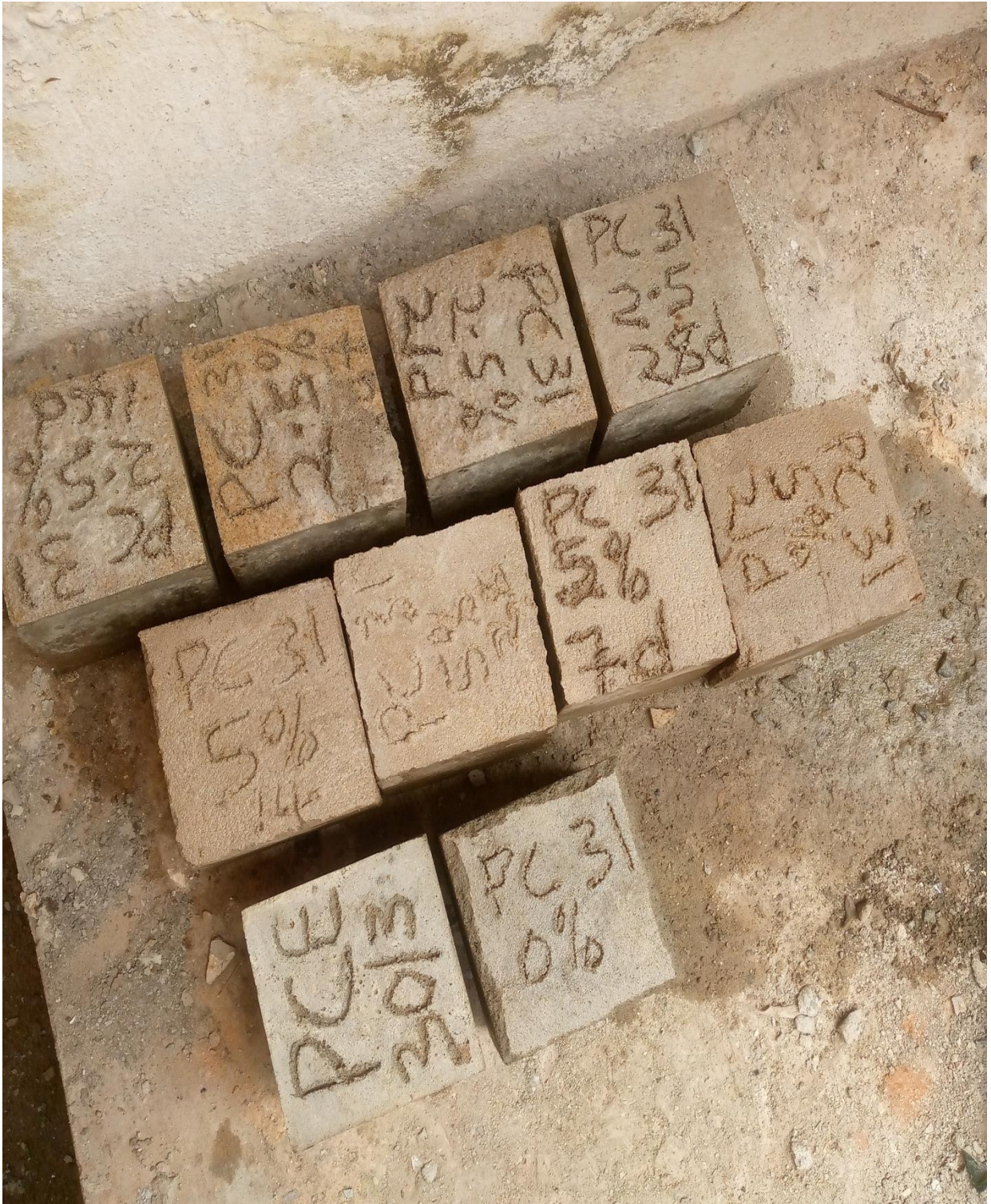
Fig 3.2: Moulded blocks in the process of curing.
