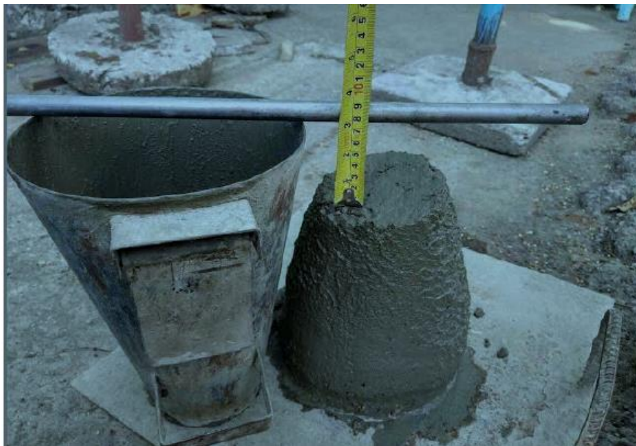
Figure 3.2 Measuring slump value
