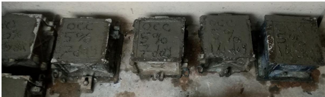
Plate 3.8 Picture of concrete cube moulds containing fresh concrete.
