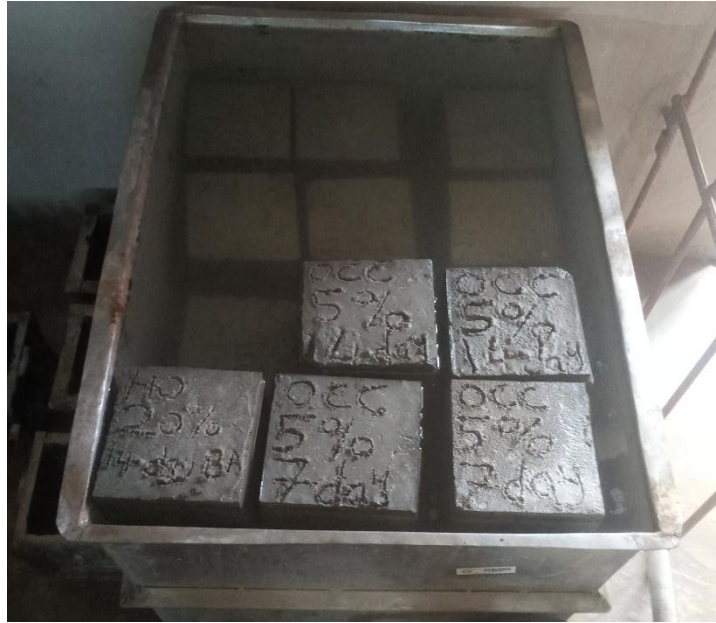
Plate 3.9 Picture of a curing tank containing concrete cubes left for curing
