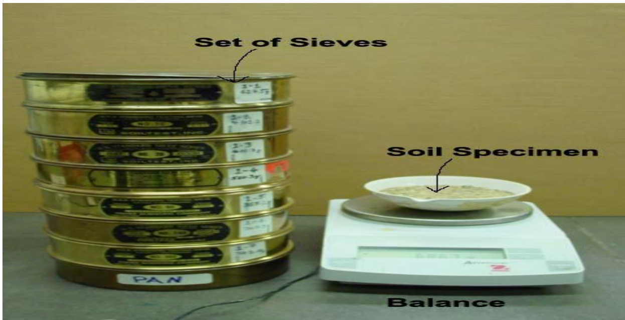
Figure 3.4 Apparatus for Particle Size Distribution Test (Sieve Analysis)
