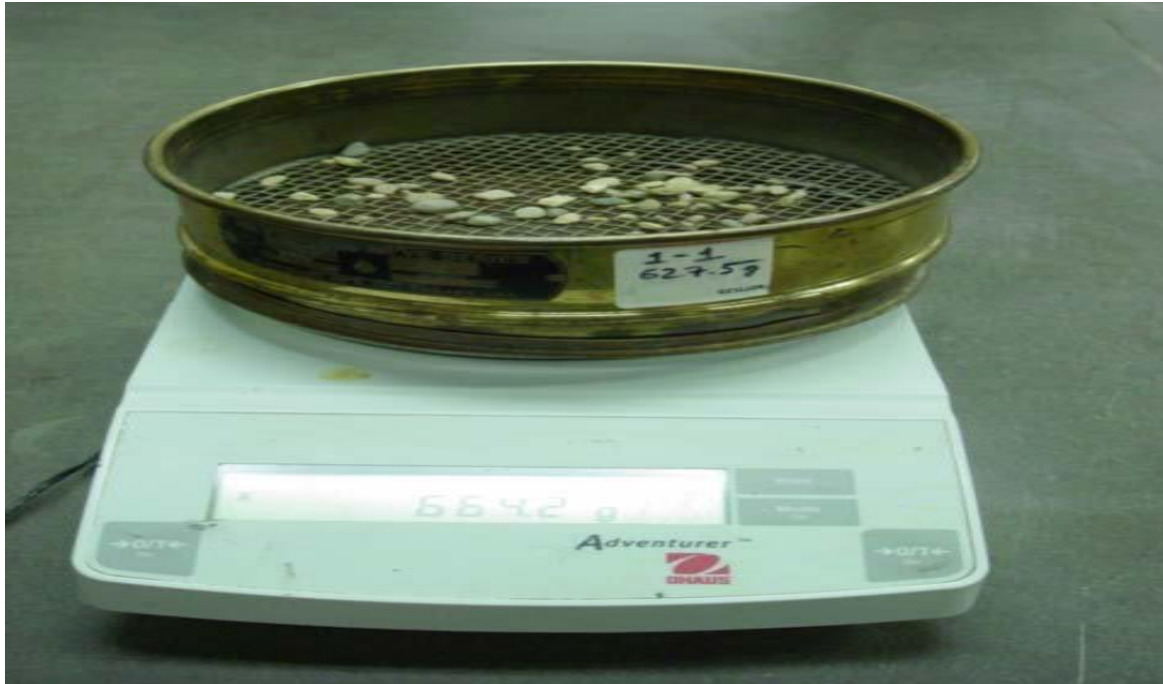
Figure 3.3 Apparatus for Particle Size Distribution Test (Sieve Analysis).
