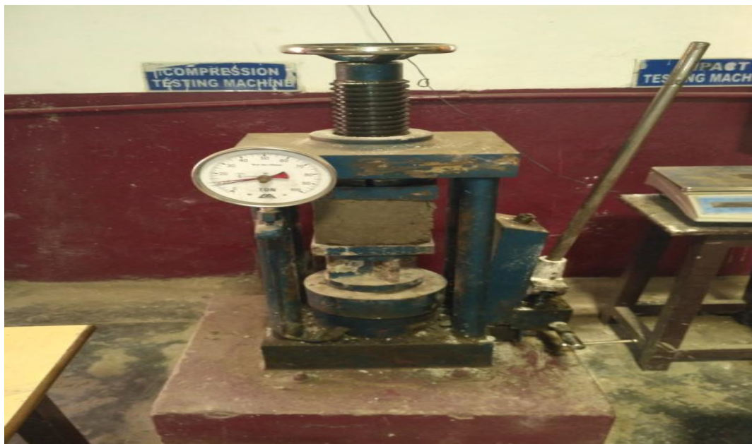
Plate 3.8: Universal Testing Machine for Compressive Strength Test
