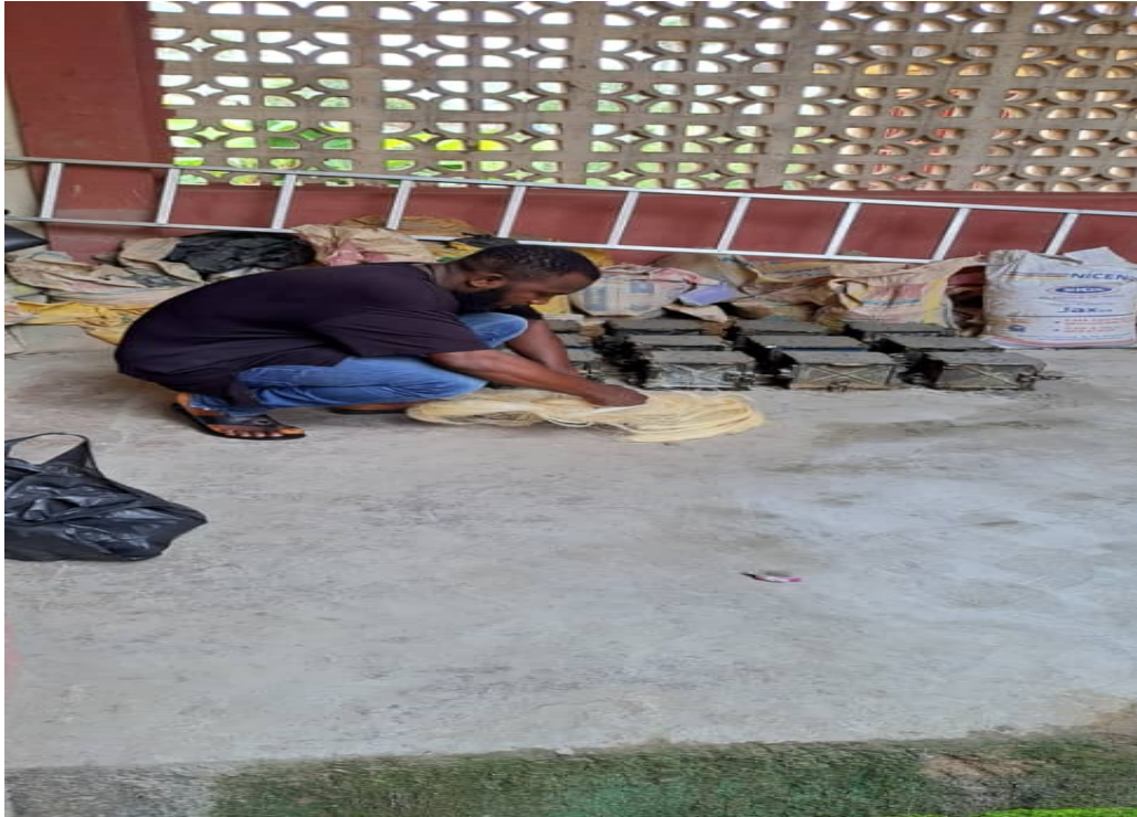
Plate 3.9: Arrangement of Kenaf Fiber used for Production of Concrete Cubes
