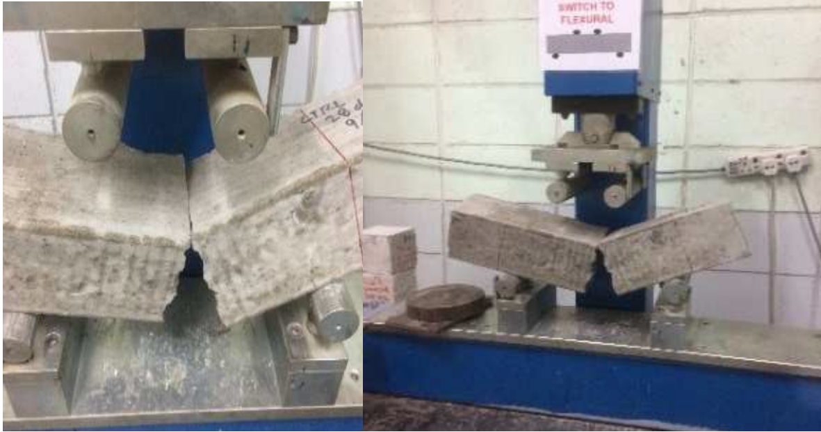
Figure 4.13: Failure Mode of Plain Concrete (Control)
