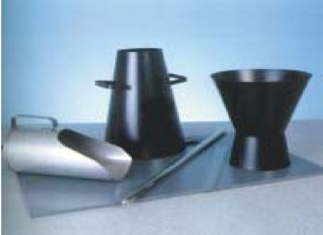
Plate 3.10: Apparatus used for Slump Test
