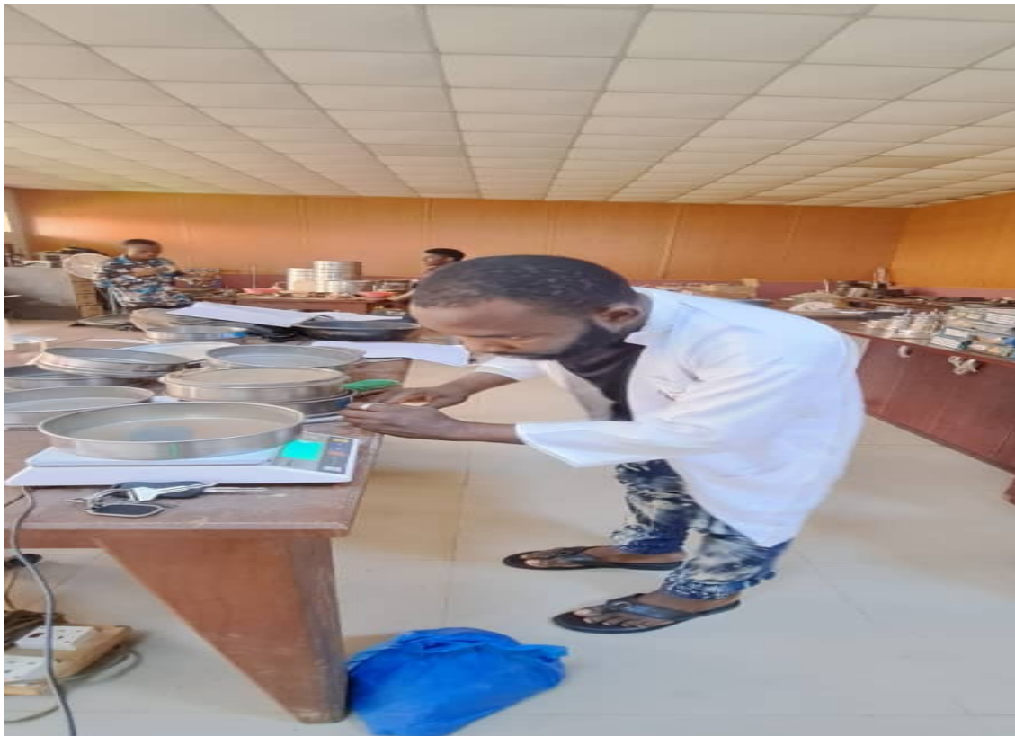
Plate 3.6: Weighing of Samples Retained on the Sieve
