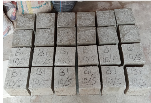
Plate 2 Cubes to be Tested for Compressive Strength
