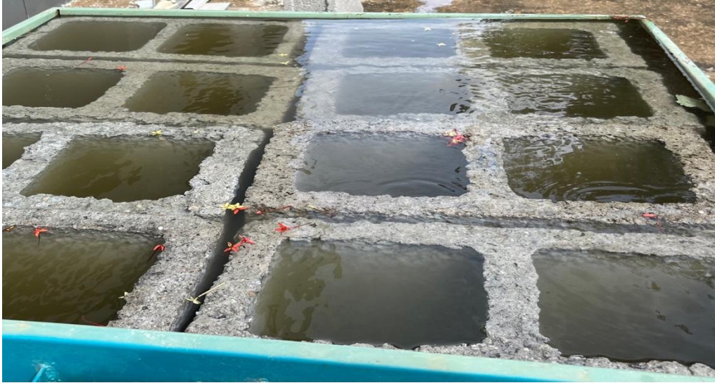
Fig. 2: Block samples submerged in water
