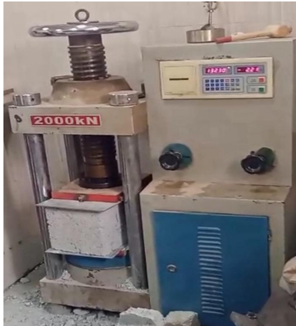
Fig. 1: Crushing a block using the Universal Compression Machine
