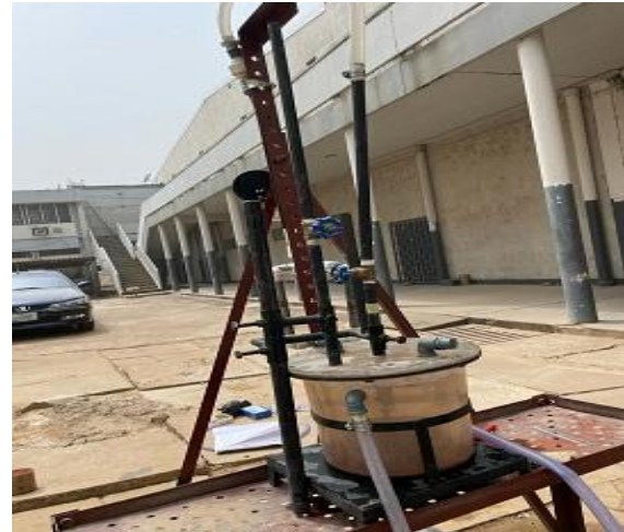
Plate I: The fabricated jet erosion test apparatus (JETa).
